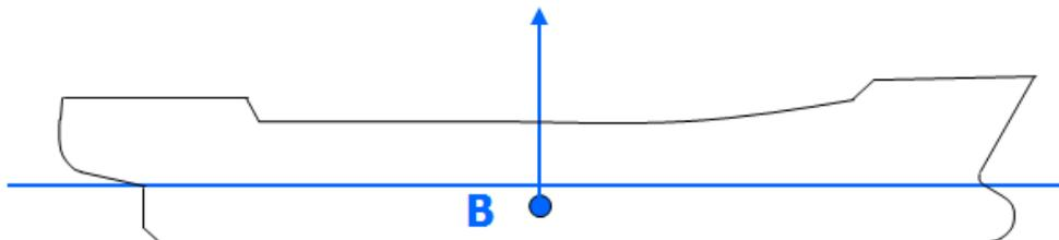
When the buoyant forces **EQUAL** the mass forces, the vessel floats.
